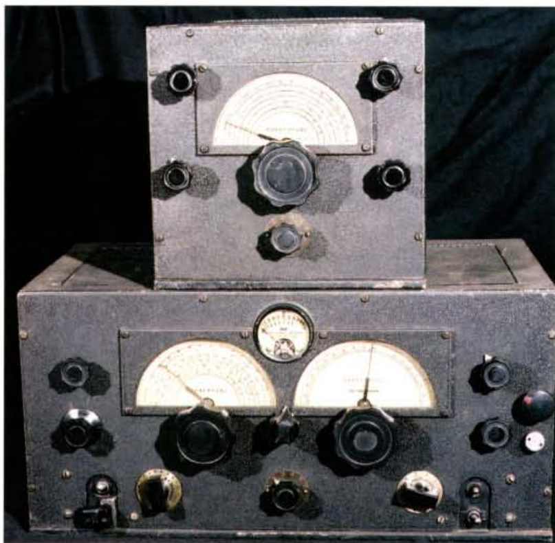
● Fig. 1: The RME-69 receiver with DB-20 preselector above. The added controls (see text) are visible on right side of front panel.
