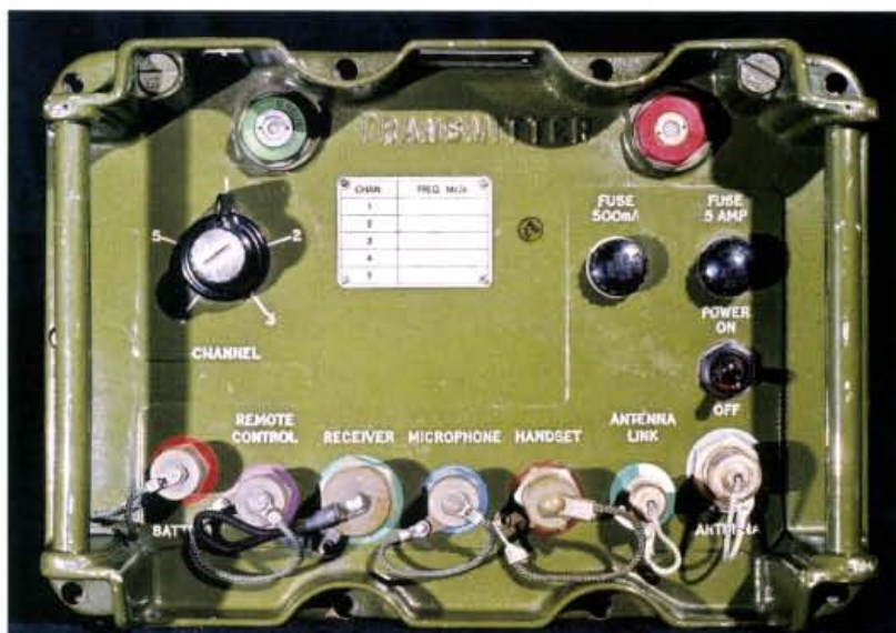
Fig. 3: The 'mystery' Transmitter Radio 5 R set with array of connectors along the bottom of the unit. In his column Ben poses the question "Can you help solve the mystery?" (see text).
