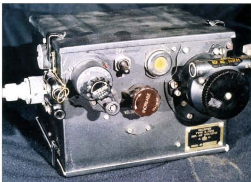
Fig. 4: The diminutive R1147B receiver, the tuning control (top right) can be driven by a Bowden cable from the control box.
