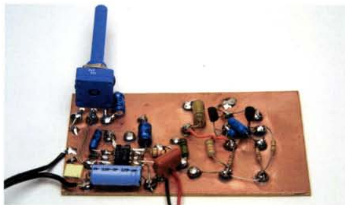
Fig. 5: One of the projects G3XFD built using the CICO system - the null detector and audio amplifier from the Radio Basics C/R Bridge, as published in the January issue of PW (see text).
