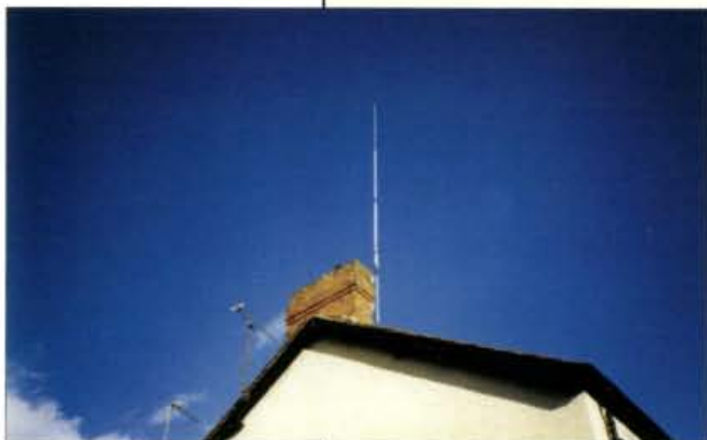
● Fig. 1: The A99 antenna assembled and mounted on the highest point of the house.
