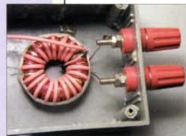
● Fig. 4: A smaller version of the G5IJ antenna toroid mounted in a suitable box, prior to weatherproofing. You can see how the antenna connections terminals are mounted.
