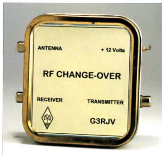
● This month G3RJV describes simple methods- including the radio frequency sensing change-over systems shown here - so you can add that extra versatility to your QRP transmitter.
