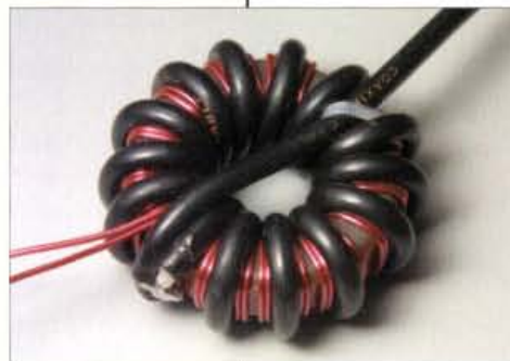
● Fig. 3: A completed transformer ready to be mounted in a box for weatherproofing purposes. The secondary (inner) winding has been wound with slightly thicker wire so, taking up slightly more room on the core.
